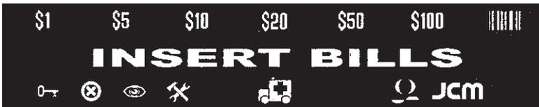
When there is a problem requiring immediate attention, a flashing blue icon of an ambulance blinks on the front of the bezel and the Bill Validator shuts down. If a red icon also lights up, this gives the slot tech more specific information about the problem. The red icons are a key, a crossed circle, an eye, and crossed hammer and wrench. The JCM logo indicates the cash box is full when lit.
